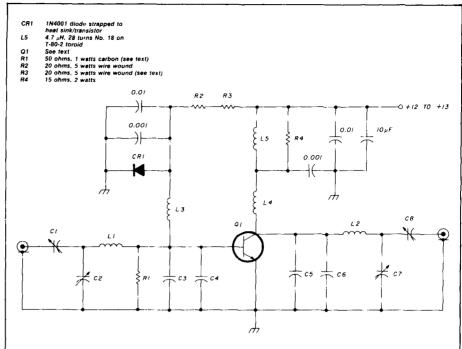
fig. 7. A typical power bipolar amplifier schematic with recommended starting values. See text for further explanation.
